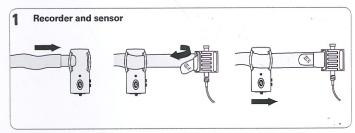
Thread the belt through the brackets of the ApneaLink Plus and the effort sensor. Fix the Velcro® fastener on the belt and move the recorder to a comfortable position.
