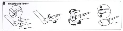
Attach the finger pulse sensor to the fourth finger on your non-dominant hand. The symbolized finger on the adhesive strip shows the position in which the strip is placed on the finger nail.
